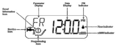
While in the "Service" position the display will alternate between time of day and days remaining till regeneration. The clock uses a standard 12 hour display.
